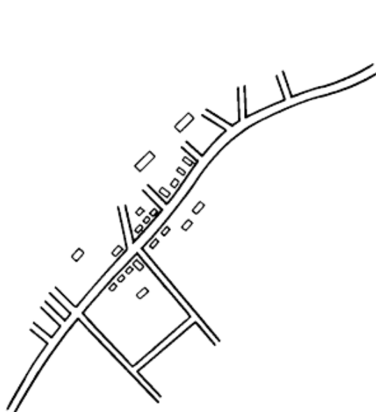
Fig 3.12 Existing interurban road results in considerable conflict between through traffic and local traffic in a Korean village (Ross Silcock Partnership)
