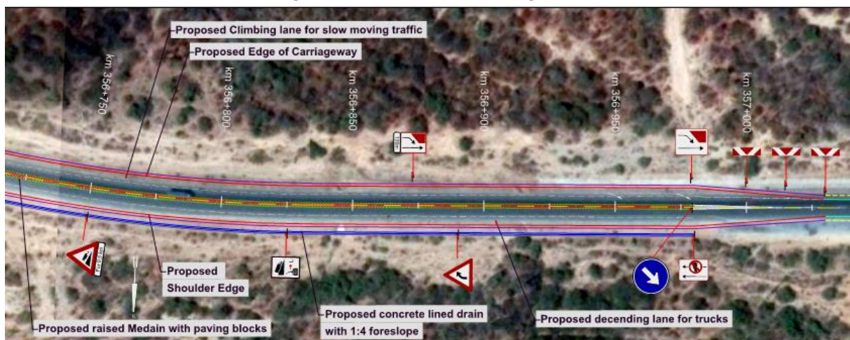
Figure 7.7.2-3: End of Climbing Lane
