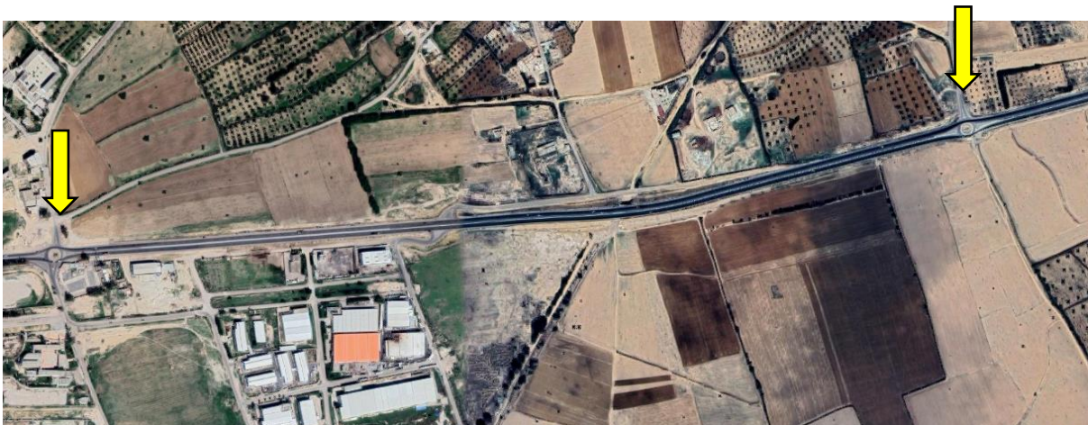
Figure 9 - Implementation of roundabouts at city entrances to moderate speeds and change the typical cross section from rural to urban areas
