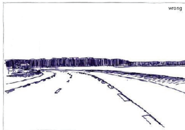
Illustration 21: Curve without setting leads to destabilisation of the driver especially in the night. [26]
