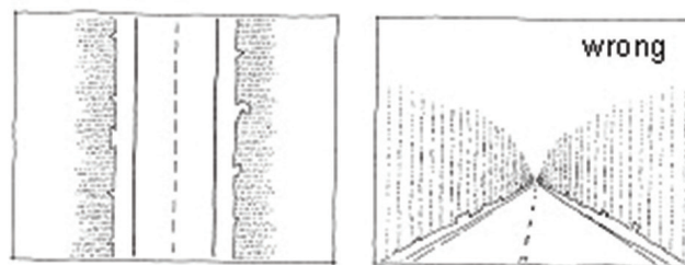
Illustration 12: Density of the field of view is low; monotonous and long straight-ahead section stimulates subconscious speeding up [11]
