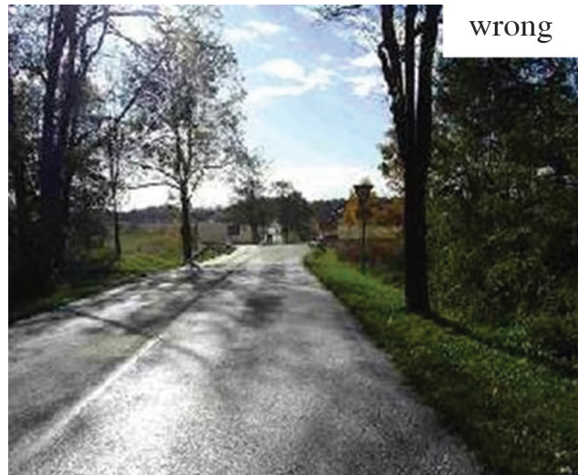
Illustration 9: Intersection not visible 125 m ahead: unexpected braking and high speed cause rear-end collisions [10]
