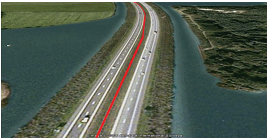
Illustration 38: Unintended distance illusion at an accident location in the Netherlands: safety barriers suddenly swing to the left. [38]
