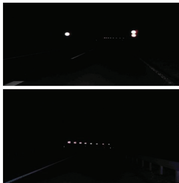
Illustration 42 :Perspective illusion: at night signs sometimes give a wrong expectation of the direction of a curve first impression left, after 100m – right. [13]
