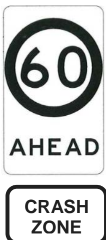
Figure 8.3: A potential design of a speed limit ahead sign with a supplementary plate
