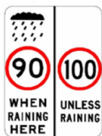
Figure 6.5: Static wet weather speed limit sign used in NSW speed limit trial
