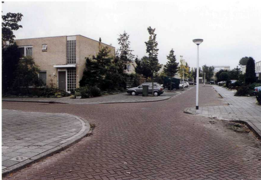
Figure 6.28 Extended sidewalk at T-intersection
