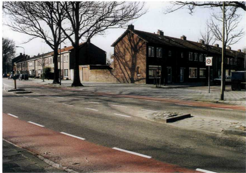
Figure 6.17 Gateway treatment Transition 50 km/h arterial to 30 km/h access road
