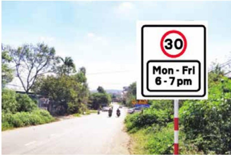
Figure 19. A time-based speed limit sign
