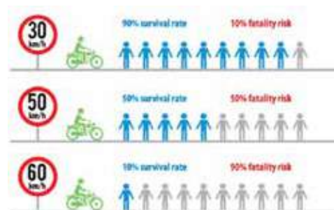
Figure 1: Probability of Fatal Injury in road crashes in relation to vehicle speed
