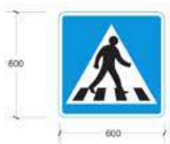
Figure 21: Specifications for sign W 43 “Pedestrian crossing location”
